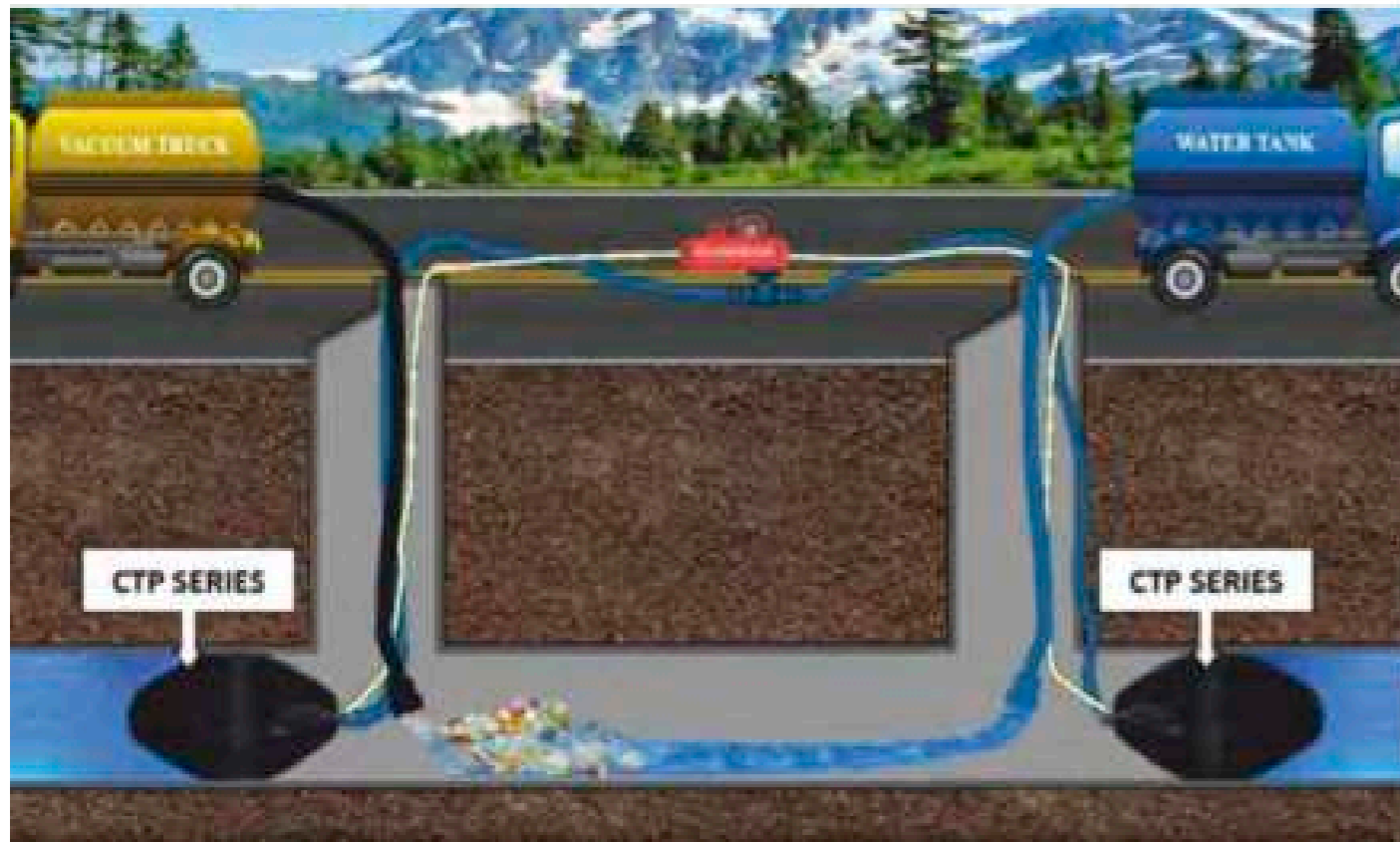
Picture-6 CTP series in pipeline water bypassing for cleaning
